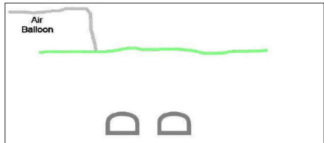
30 metre deep cutting at the Air Balloon Inn vs. Dual tunnel type bridge underneath its car park
